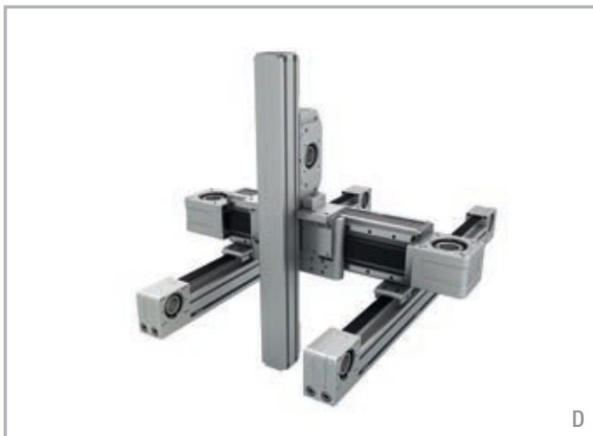
D - Linear units: X Axis 2 E-SMART - Y Axis 1 R-SMART - Z Axis 1 S-SMART Connection kit: 2 fixing brackets Kit for 2 R-SMART (Y axis) on 2 E-SMART (X axis). Connection plate Kit for S-SMART (Z axis) on 2 R-SMART (Y axis). Parallel Kit
